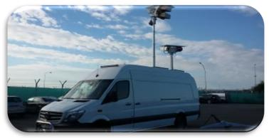
Mobile Surveillance Units (SUV): Equipped with day/night (Flir) camera
